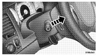
High Beam/Low Beam WINDSHIELD WIPERS AND WASHERS The multifunction lever is located on the left side of the steering column.
